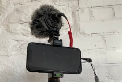
A shotgun mic is directional and useful for recording when the sound source is further away.
